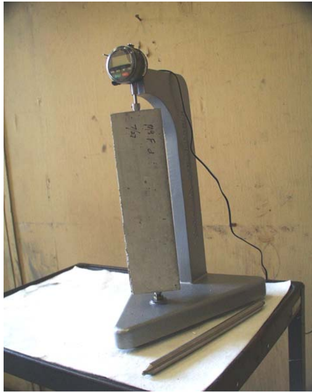
Figure 3-2 Length reading taken with length comparator
