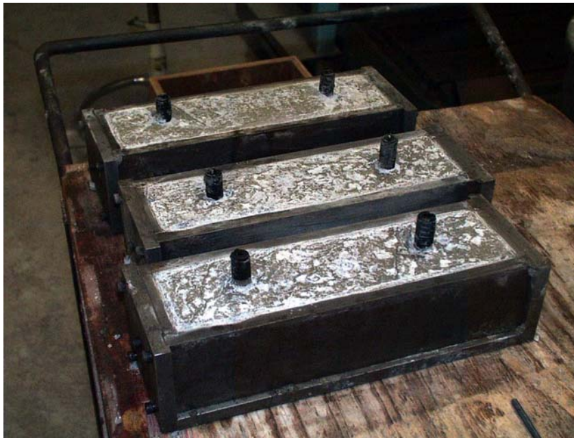
Figure 3-1 Specimens in molds
