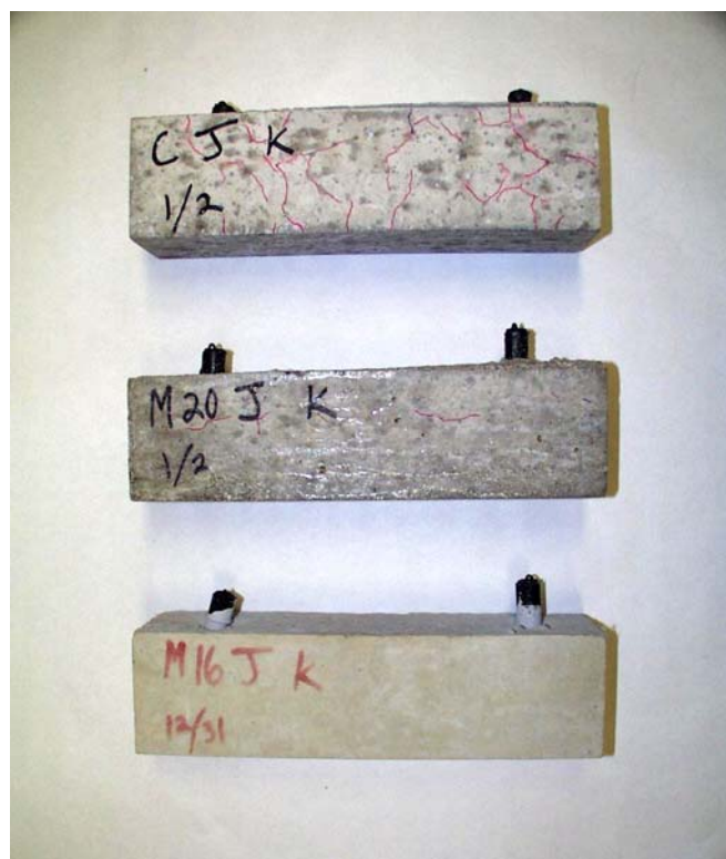
Figure 5-2 Sketches of cracks on specimens of wet/dry series
